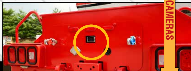
Rear viewing camera
